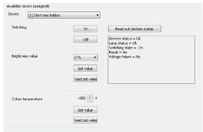
Figure 80: Device-orientated DALI test environment
