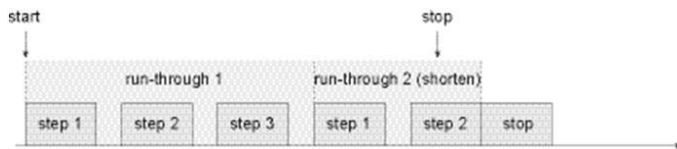
Figure 57: Example of an effect sequence with manual stop (here: 3 effect steps, run-through 2 is stopped early)
