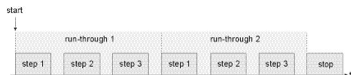
Figure 56: Example of an effect sequence with automatic stop (here: 3 effect steps, 2 run-throughs)
