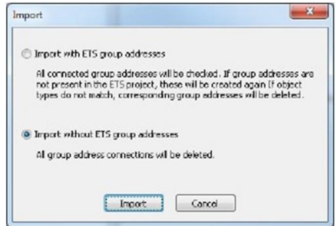
Figure 23: Import dialog to select an import with or without KNX group addresses
