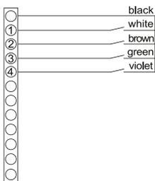
**Schema di collegamento PB44A01DL2****Wiring diagram PB44A01DL2**
